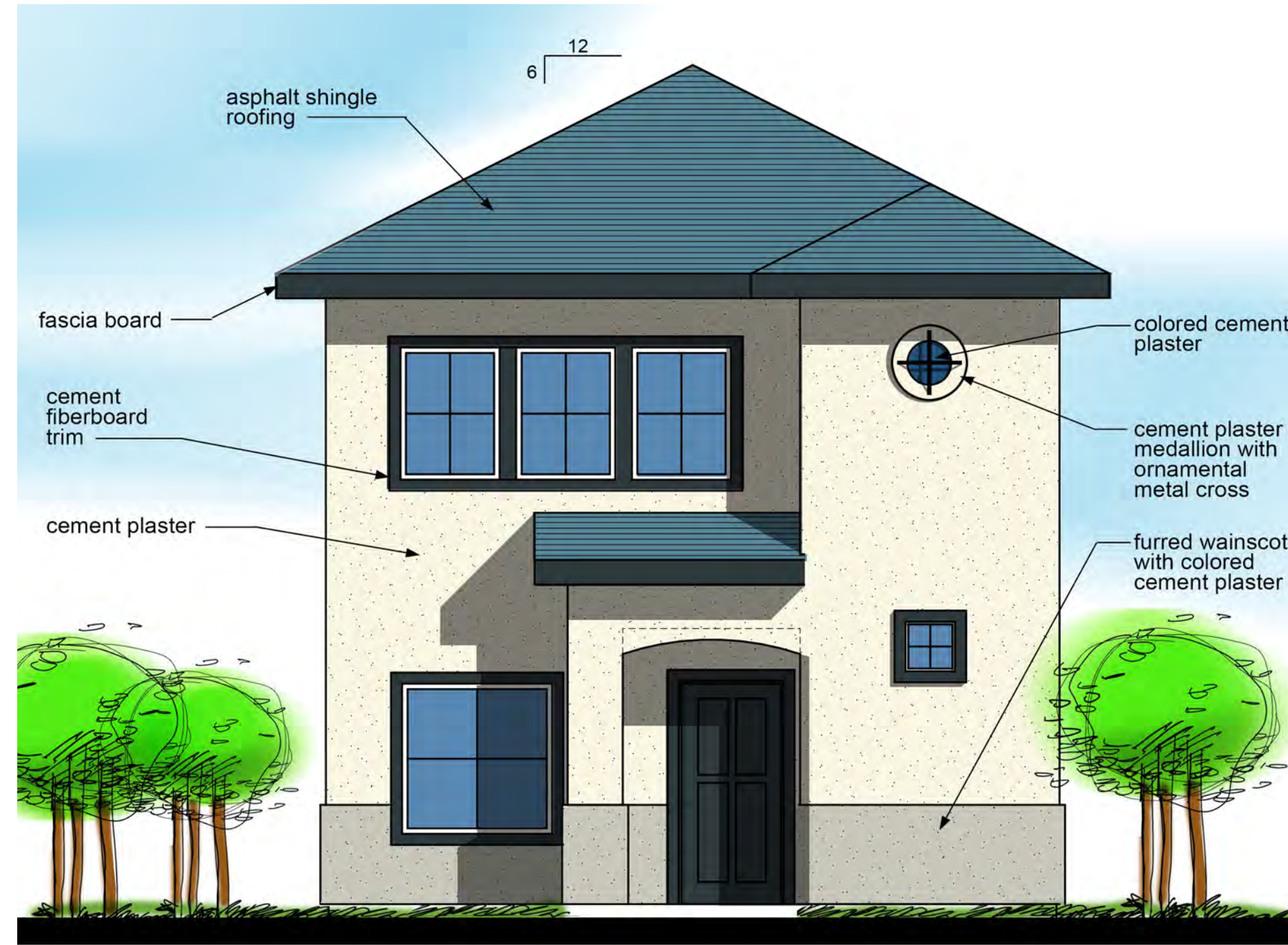
C1 RENDERED ELEVATION 1 SCALE: 1/4" = 1'-0"
