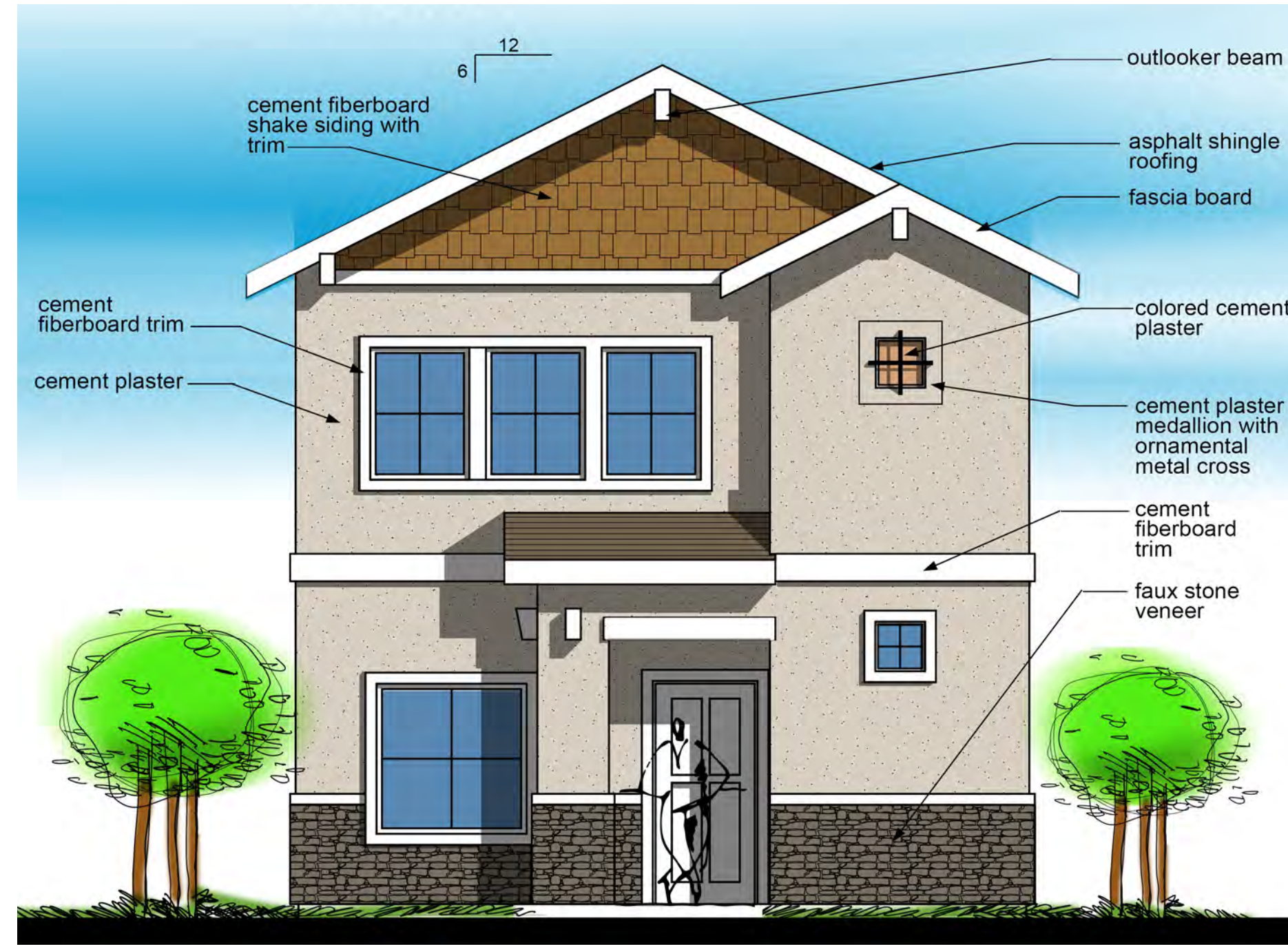
C1 RENDERED ELEVATION 2 SCALE: 1/4" = 1'-0"
