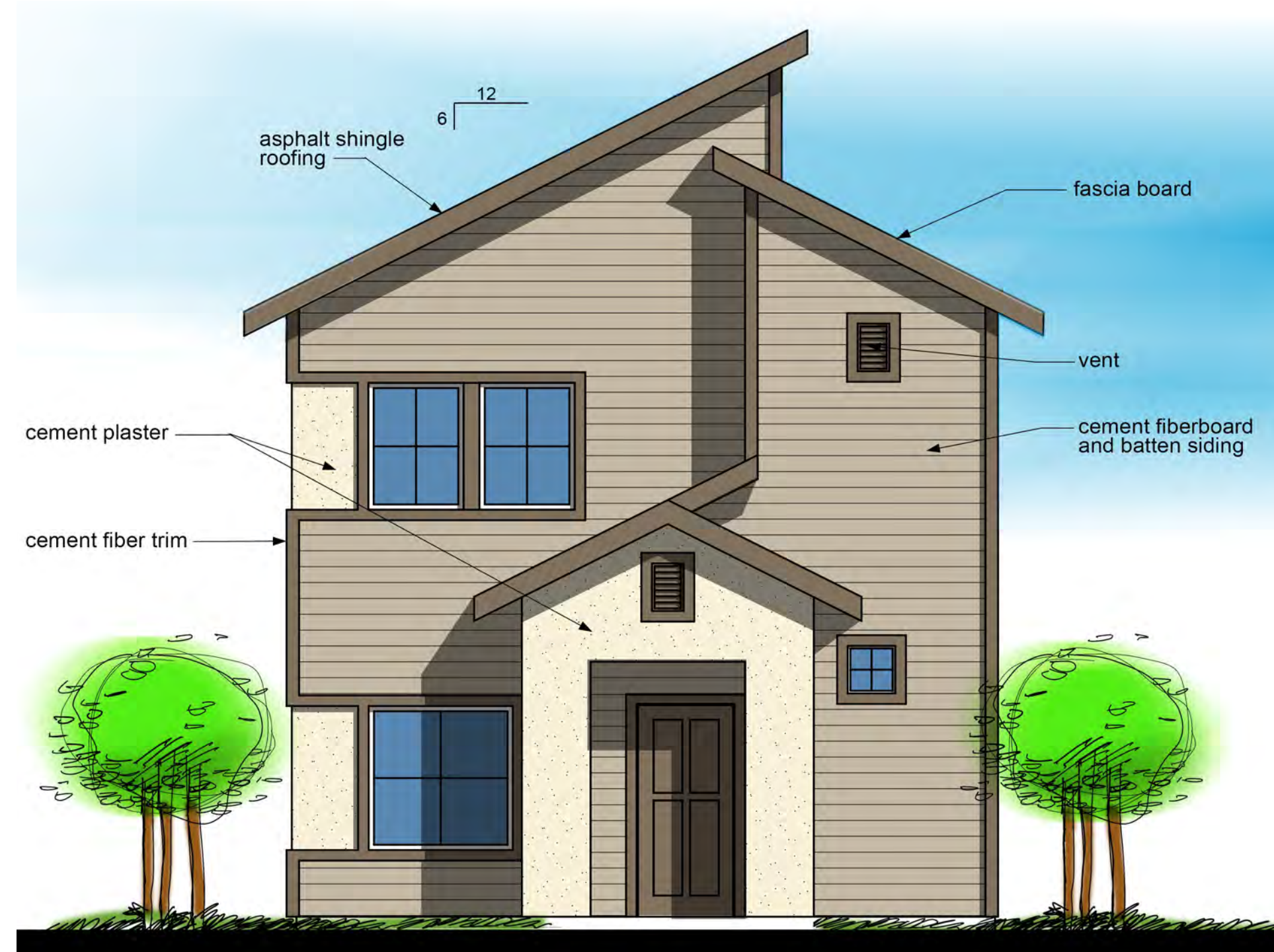
C1 RENDERED ELEVATION 3 SCALE: 1/4" = 1'-0"
